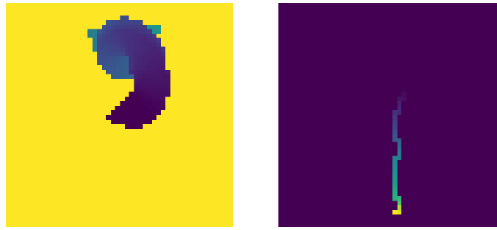
(a) Two voxel grid maps maintained in [3]. The left is the “Last Time Observed Map” t_i ; Darker color means the voxel is observed more recently. The map on the right is the “Future Occupancy Map” v_i . The future trajectory is projected onto the map. The darker color means the MAV will occupy the voxel in the nearer future.
